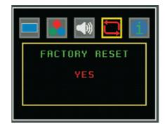
Select YES to return to the factory setting. Factory setting on display is at 1024 x 768@60Hz with full size screen, Color setting's factory default rate are as the value in the bracket n the OSD chart and SDI audio is on auto.
