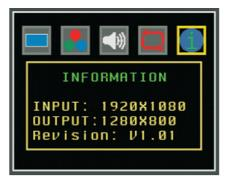
Displaying both input source and output display timing with software firmware version.
